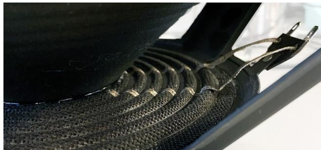
*Figure 4: Voice coil lead out wires are attached to the spider for highest reliability at even high excursions*
