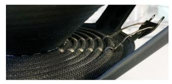
Figure 4: Voice coil lead out wires are attached to the spider for highest reliability at even high excursions
